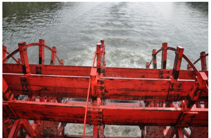
The General Jackson Showboat had a single paddle wheel mounted at the fantail
